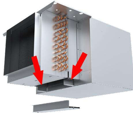
**Step 4:** Lift Electric Heat Rack Upwards to Disengage From Internal Support Brackets. Tilt Rack Towards Coil, Angling Electric Heat Rack Downward and Out of the Heater Access Compartment.
