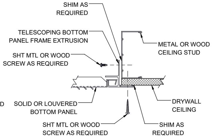
NOTE: CEILING "T" BAR GRID MAY NOT SUPPORT TELESCOPING BOTTOM PANEL ASSEMBLY. BOTTOM PANEL ASSEMBLY MAY REQUIRE INDEPENDENT SUPPORT.
