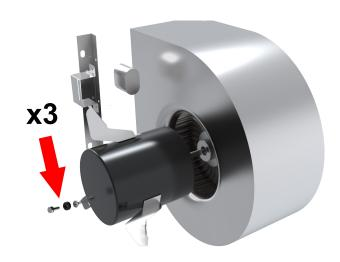
Example 1: Exploded Motor and Blower Illustration (Cap Screws, Grommets, and Inserts are Typical x3)
