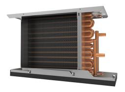
The sloped, insulated drain pan can be equipped with a secondary drain connection. Standard drain pans are externally insulated, single wall galvanized steel. The drain pan is easily removable for cleaning. The optional auxiliary drip pan to catch condensed moisture from valves and piping is easily attachable to the drain pan. Care must be taken to ensure that the unit drain pan does not slope away from the outlet connection.
