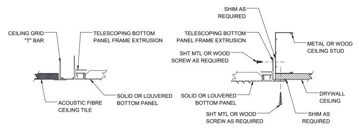
NOTE: CEILING "T" BAR GRID MAY NOT SUPPORT TELESCOPING BOTTOM PANEL ASSEMBLY. BOTTOM PANEL ASSEMBLY MAY REQUIRE INDEPENDENT SUPPORT.
