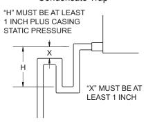
Trap detail for positive cabinet static pressure
