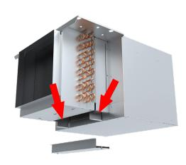
Step 4: Lift Electric Heat Rack Upwards to Disengage From Internal Support Brackets. Tilt Rack Towards Coil, Angling Electric Heat Rack Downward and Out of the Heater Access Compartment.
