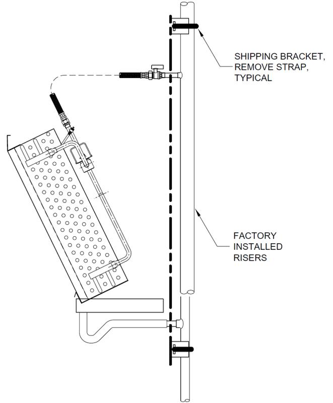
**FIG 4 - FACTORY INSTALLED RISERS, Primary/Secondary CONFIGURATION**
