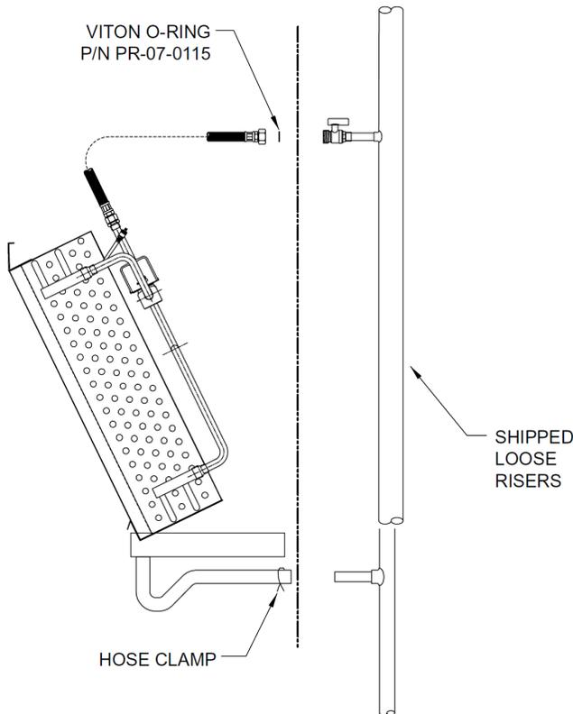
**FIG 6 - FACTORY FURNISHED, FIELD INSTALLED RISERS, Primary/Secondary**
