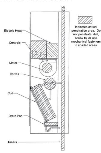
Due to factory manufacturing tolerances and job site construction variations, some unit casing surface conditions may exist that could require additional framing or shimming of the finished wall surface. ALL WORK REQUIRED TO ACHIEVE THE DESIRED FINISHED WALL SURFACE CONDITION IS THE RESPONSIBILITY OF OTHERS.
