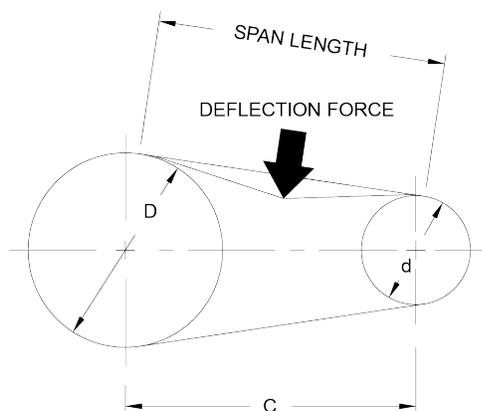
1. Measuring belt span. Lay a tape measure along the top of the belt, measure between the points at which the outside of the belt meets the outside of the sheaves. The following formula can be used to calculate the belt span.
