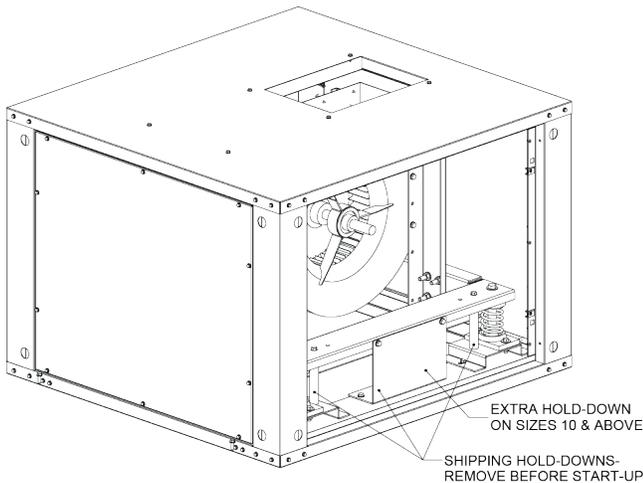
**FIGURE 9 - ISOLATOR INSTALLATION**
