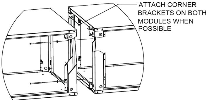
**FIGURE 4 - ASSEMBLY, UNITS WITH BASE RAILS**
