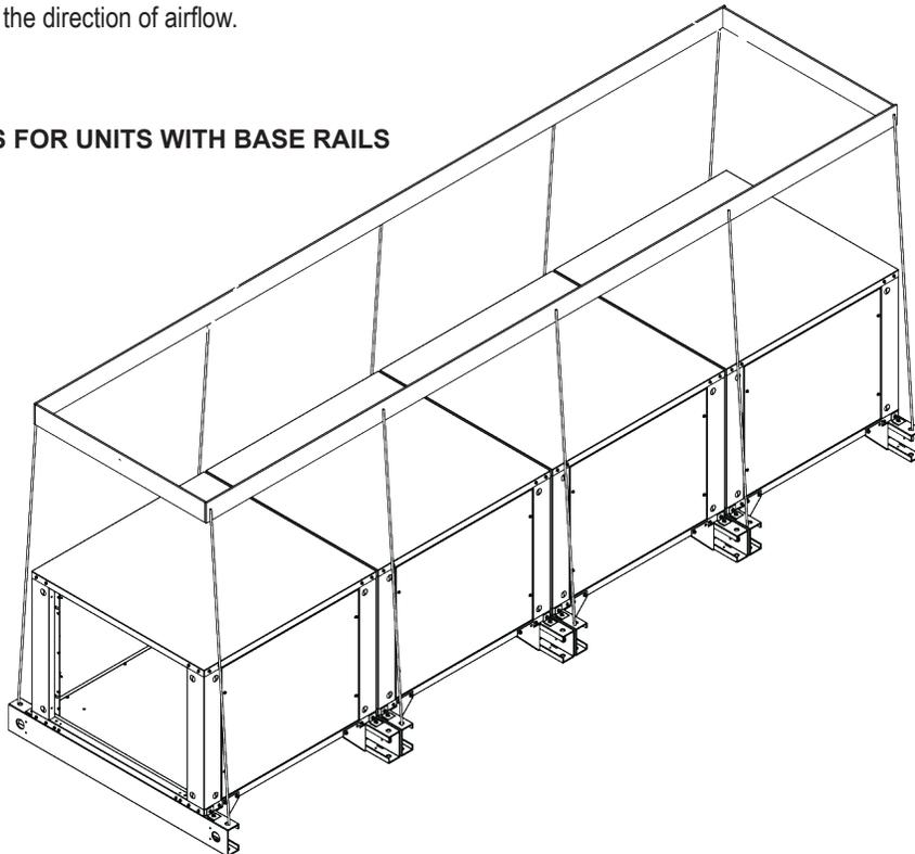
Units with base rails can be rigged by means of lifting holes on the end of base rail (see Figure 1 on page 5).
