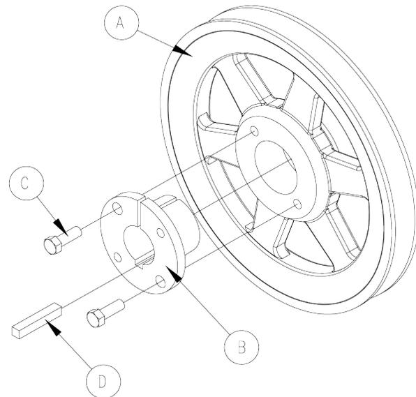
10. Be sure that all keys are in place. Be sure that all setscrews and capscrews are torqued properly before starting drive. Check setscrews and belt tension after 24 hours of service.
