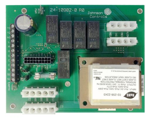
Figure F.1: Fan Relay Board (FRBii)
