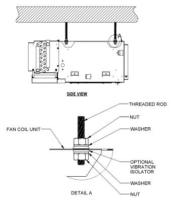
Figure 1: Typical ceiling installation
