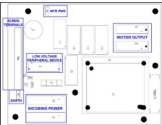
Figure F.2 – Connector layout
