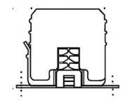
Figure 10 Current Switch mounting
