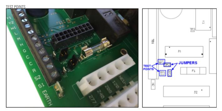
Figure F.3: FRBii Jumpers and Test Points
