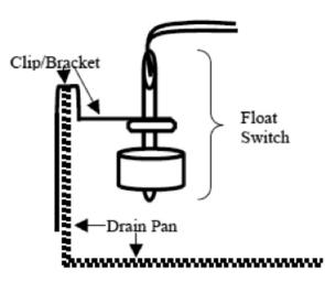
Figure 15b: Drain pan float switch diagram
