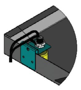
Figure 15a: Drain pan float switch installed
