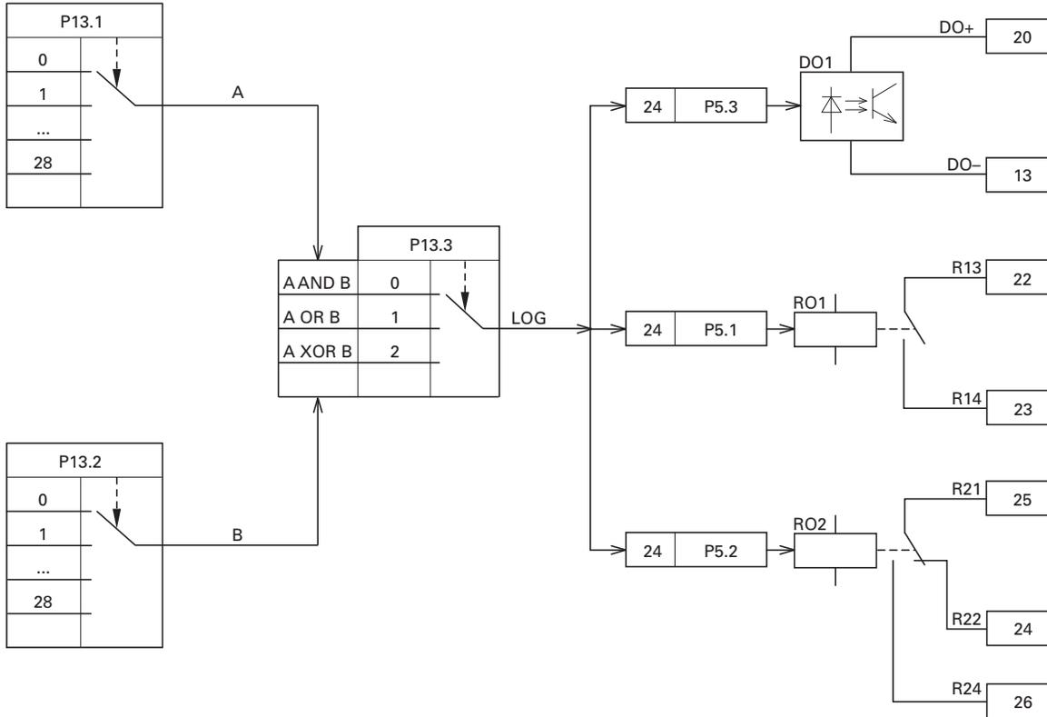
**Example:** Digital output RO1 (N/O contact R13/R14) is required to indicate during operation that the set current limit has been reached:
