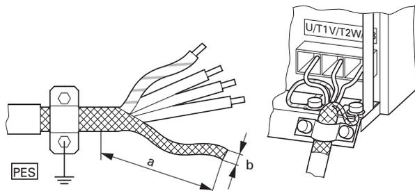
Twisted shielding braid should be connected with a ring cable terminal (see figure on **Page 31**) on PES.
