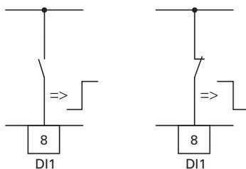
In the factory setting, the operation of the VSM II is active via control signal terminals (I/O) with LOGIC+ (Source type):
