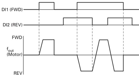
The start enable via control signal terminal 8 (DI1) is always required for operation:
