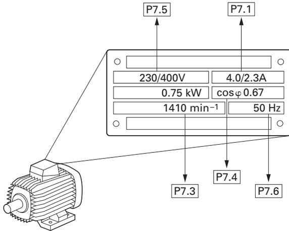
The motor data is set to the rated operation data for the frequency inverter and depends on the performance variables in factory settings.
