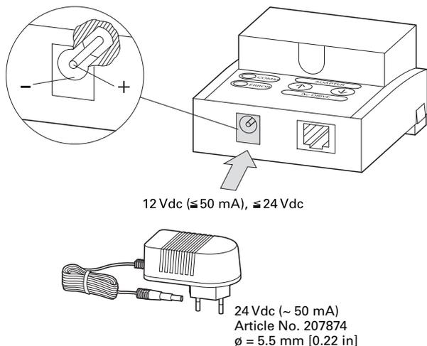
The VSM2-PCADAPTER can also be fed with a 12 to 24 Vdc external power supply. The connection is implemented using a 5.5 mm power supply plug.
