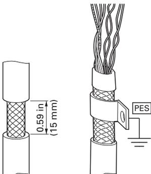
As an alternative, in addition to a broad area cable clip, you can also twist the shielding braid at the end and connect to protective ground with a cable clip. To prevent EMC disturbance, this twisted shielding connection should be made as short as possible (see figure on **Page 33**).
