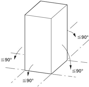
An installation that is turned by  $180^\circ$  (stood on its head) is not permitted.
