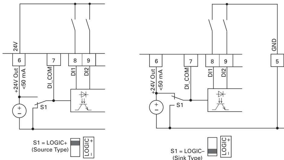
Source type (LOGIC+) = switch at the voltage source. All digital inputs are connected to the voltage sink via microswitch S1 (0V = reference potential GND).
