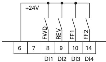
The fixed frequencies FF1 = 10 Hz, FF2 = 15 Hz and FF3 = 20 Hz can be called via digital inputs DI3 (control signal terminal 10) and DI4 (control signal terminal 14) in the factory setting.
