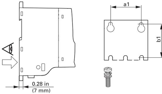
Install the screws in the specified positions first. Then set the frequency inverter on the prepared wall-mount and tighten all screws.
