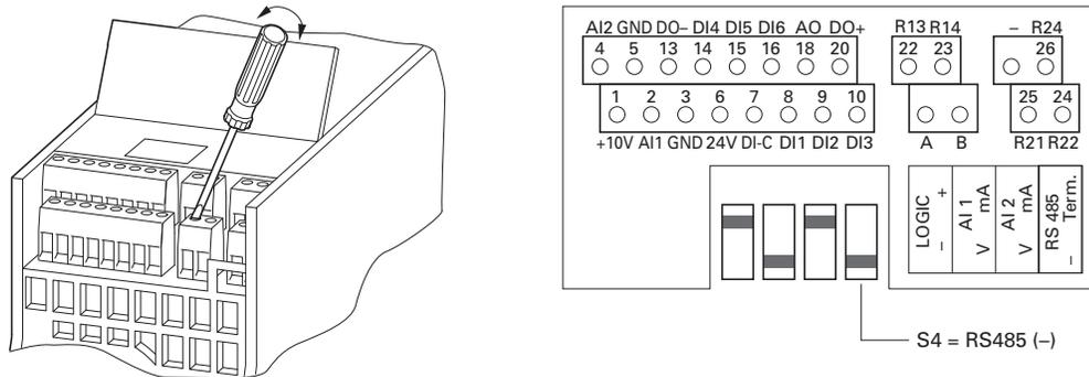
The two control signal terminals A and B enable the connection of a shielded RS485 twisted-pair cable.
