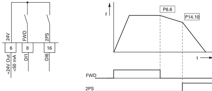
The Stop function with deceleration time can be activated with parameter P6.8 = 1. If the enable signal on the digital input DI1 (FWD, control signal terminal 8) is switched off, the output frequency of the frequency inverter can be reduced according to the deceleration time (dec1) set at P6.6.
