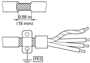
Shielded, four-wire cable is recommended for the motor cables. The green-yellow line of this cable connects the protective ground connections from the motor and the frequency inverter and therefore minimizes the equalizing current loads on the shielding braid.
