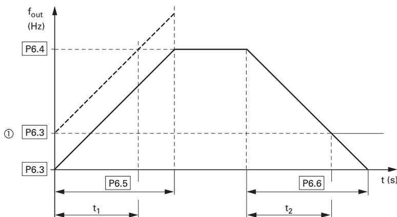
The values for the acceleration time  $t_1$  and the deceleration time  $t_2$  are calculated as follows:
