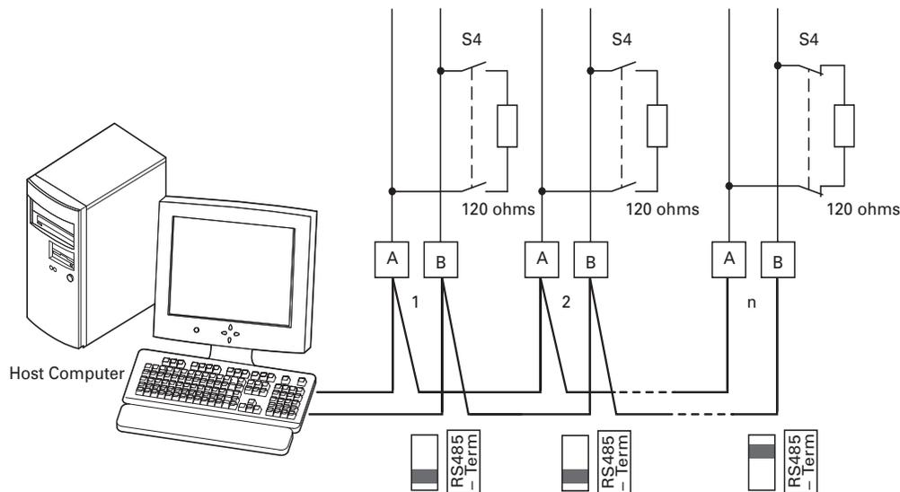
The figure shows a typical arrangement with a host computer (master) and any number (maximum 31 slaves) of frequency inverter VSM II (slaves). Each frequency inverter has a unique address in the network. This addressing is executed individually for each VSM II via system parameter S2.3 and is independent of the physical connection (position) in the network.
