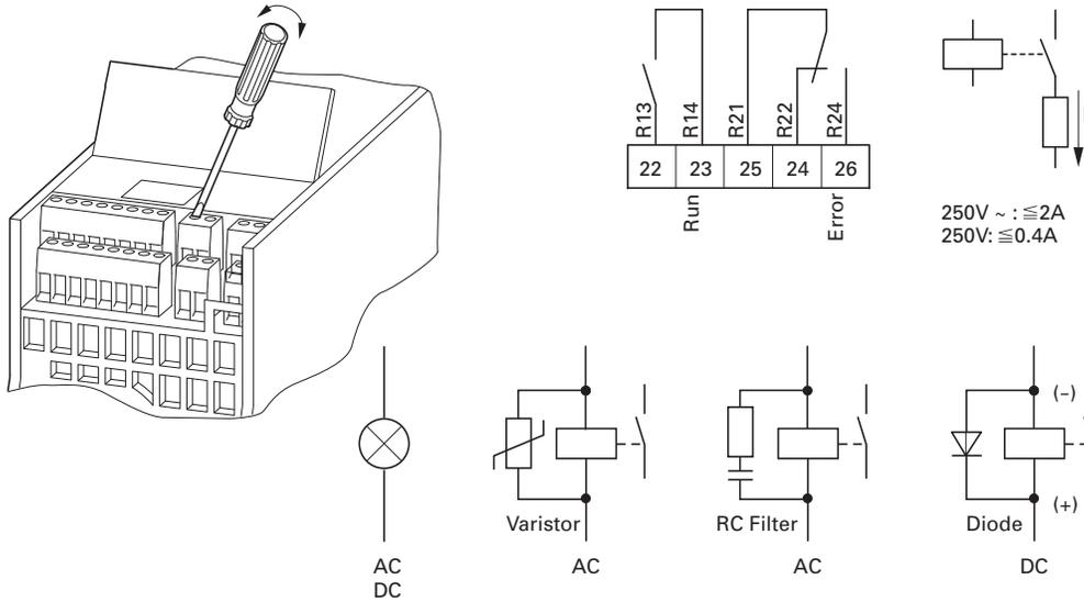
The two relay outputs (control signal terminals 22 to 26) enable the frequency inverter to generate galvanically isolated feedback signals in control circuits with other potentials:
