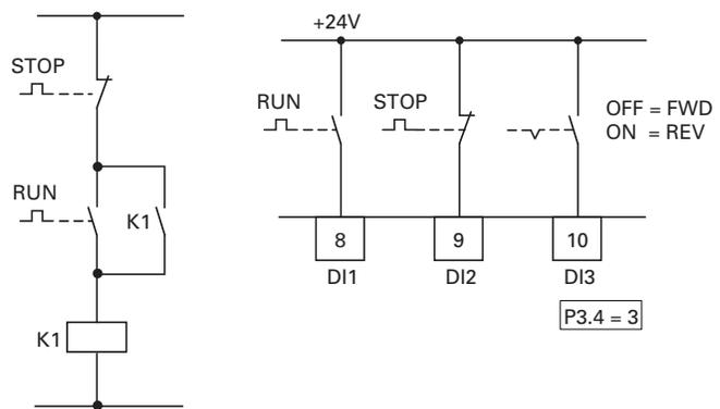
Standard actuation for a drive with pushbutton switch (Normally open, Normally closed) and self-actuating.
