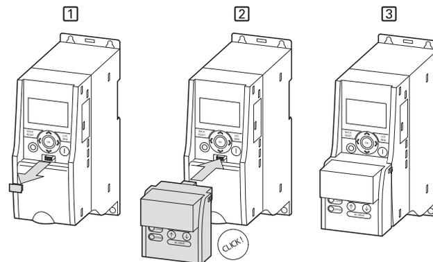
1. Remove the interface cover on the frequency inverter (do not discard)
