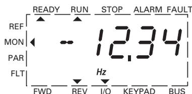
You can now set the output frequency (0–60 Hz) and therefore the speed of the connected AC motor (0– $n_{motor}$ ) with the setpoint value potentiometer via terminal 2 (proportional voltage signal 0–10V). The change in output frequency here is delayed based on the specified acceleration and deceleration ramps. In the factory settings, these times are set to 3 seconds.
