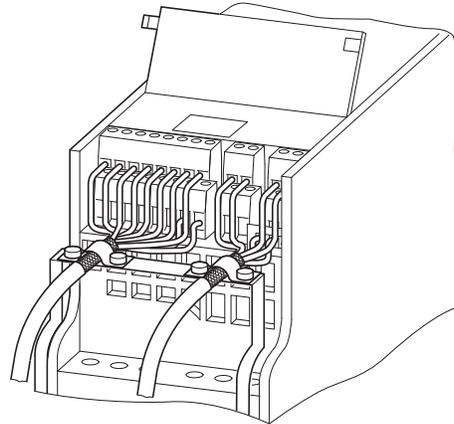
Prevent any unraveling on the other end of the control line with a rubber grommet. The shielding braid is not to make any connection with protective ground here because this would cause problems with an interference loop.
