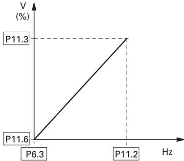
Characteristic Curve: V/Hz (P11.1) Linear
