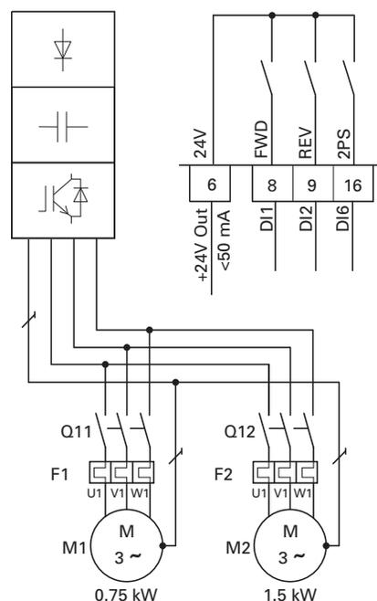
For alternating operation (rotary movement “exclusive or” of the transport rollers) on the rotary table, a frequency inverter for the largest connected load (VS4D3403B-M\_) was selected.
