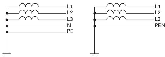
While planning the project, consider a symmetrical distribution to the three external conductors, if multiple frequency inverters with single-phase supplies are to be connected. The total current of all single-phase consumers is not to cause an overload of the neutral conductor (N-conductor).
