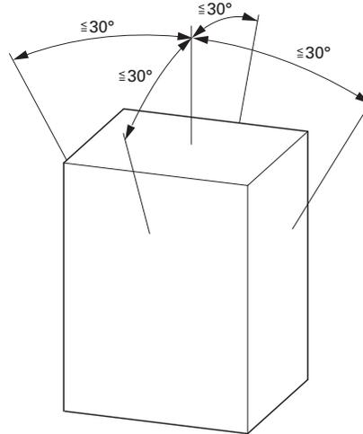
An installation that is turned by  $180^\circ$  (stood on its head) is not permitted.
