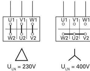
**Example:** Single-phase connection of the VS4D8204B-M\_ frequency inverter to a input voltage of 230V. The stator winding of the motor is connected in a delta circuit (motor rated current 4A as per nameplate in figure on this page).
