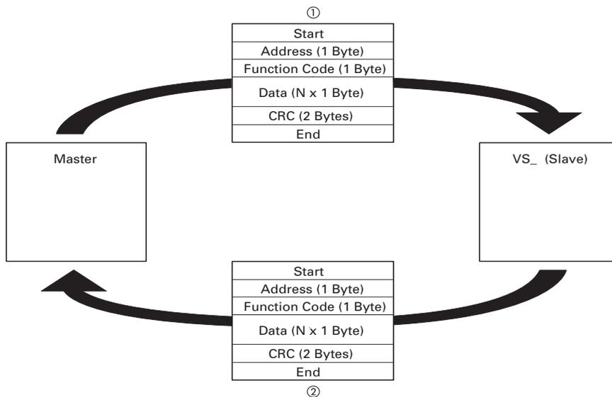
The frequency inverter (slave) only sends a response if it has received a request from the master beforehand.
