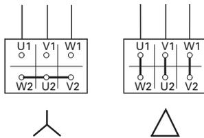
The three-phase motor with the rating plate based on the figure shown above, can be run in a star or delta connection. The operational characteristic curve is determined by the ratio of motor voltage and motor frequency, in this case.
