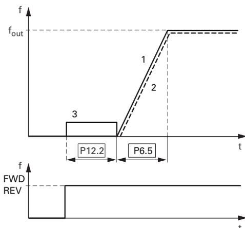
After the time set has elapsed, the frequency inverter starts automatically with the acceleration time set at P6.5. The speed of the motor [2] follows the characteristic of the output frequency [3]
