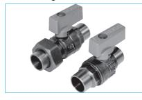
Ball valves shall be manufactured of brass OT58-UNI-5705-65 with a chrome plated brass ball with Teflon<sup>b</sup> seals. The shaft shall be sealed via dual VITON O-rings and capable of operating at 325°F and 600 psi pressure WOG. All ball valves shall be supplied with a memory stop actuator and be located in the inlet pipes to the fan coil unit.
