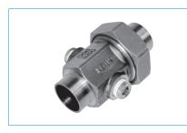
Unions shall be of forged brass ASTM B283 with VITON O-rings installed in the return and supply CW and/or HW pipes to facilitate the connection or removal of the unit.
