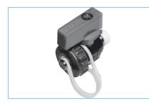
Coil blow down drain valves shall be of the chromed plated ball type with Teflon<sup>b</sup> seals; dual VITON O-rings seal suitable for operation up to  $325^{\circ}$ F and 600 psi pressure WOG. Valve connections shall be ¼-inch MNPT and  $^{3}$ ₄ inch hose bib and cap. Blow down valves shall be installed at the lowest point of the coils to enable the evacuation of all water for system repairs and/or coil replacements.
