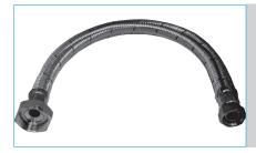
Pipe flexible connectors shall be fire rated in compliance with ASTM E 84-00 (NFPA 225, ANSI/UL 723 and UBC 8-1) with the following features: Operating pressure 400 psi @ 265°F, fittings made of brass with NPSM swivel w/ seal and MNPT; fabric reinforced EPDM core; stainless steel braid reinforcement; brass OT58 fittings; stainless steel ferrule; fiber EPDM gasket.
