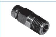
Pressure and temperature test plugs shall have  $\frac{1}{4}$ -inch MNPT thread, suitable for operation up to  $325^{\circ}$ F and 1000 psi pressure. Test plugs shall be located in the return and supply CW and/or HW pipes to measure unit total pressure drop and/ or unit water in/out temperatures.
