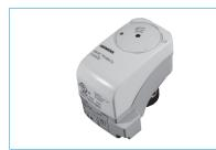
Modulated actuators shall be suitable for 24V control voltage and a signal voltage of 0-10V; UL listed for plenums to UL 873; cUL certified to Canadian Standards C22.2 No 24-93; direct coupled installation without tools; manual override; visual position indication; 40 sec max running time; <sup>1</sup>/<sub>10</sub>-inch nominal stroke; 24lb nominal force; Operation temperature between 41 and 122°F.
